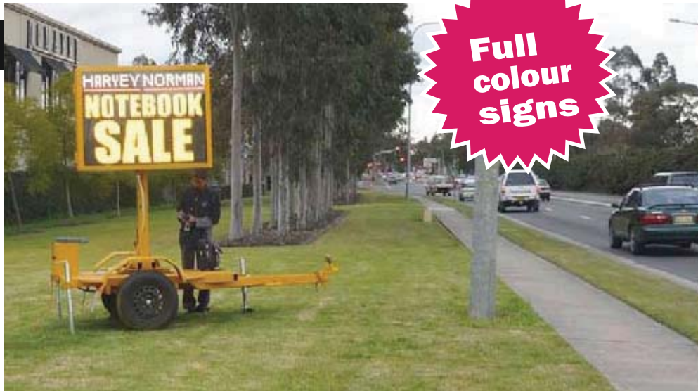
(VMS) on trailer – Size: 0.975m x 1.3m - Viewing area: 1.27sq.mtr (VMS) on trailer – Size: 1.45m x 1.95m - Viewing area: 2.86sq.mtr
